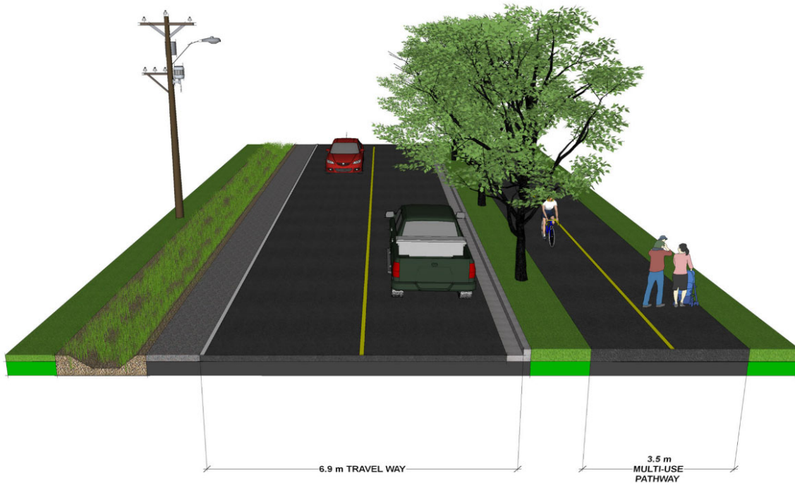
Figure 3-14: Typical Multi-Use Pathway Cross-Section
