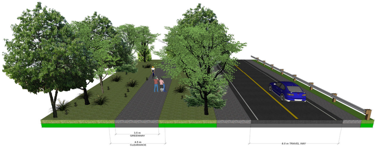
Figure 3-4: Typical Off-Road Greenway Cross-Section
