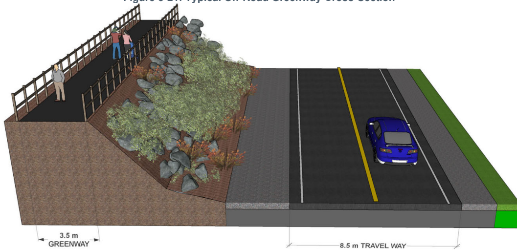
Figure 3-22: Typical Off-Road Greenway with Fencing Cross-Section
