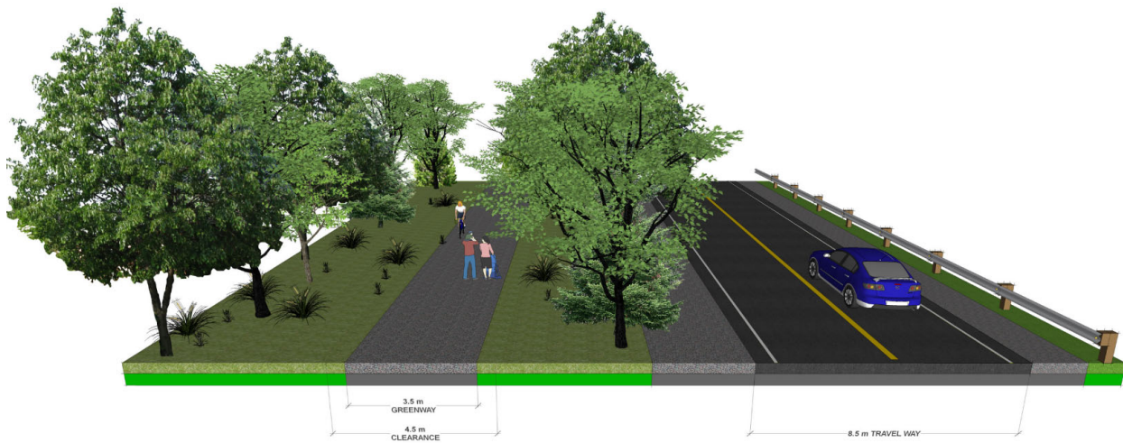
Figure 3-11: Typical Off-Road Greenway Cross-Section
