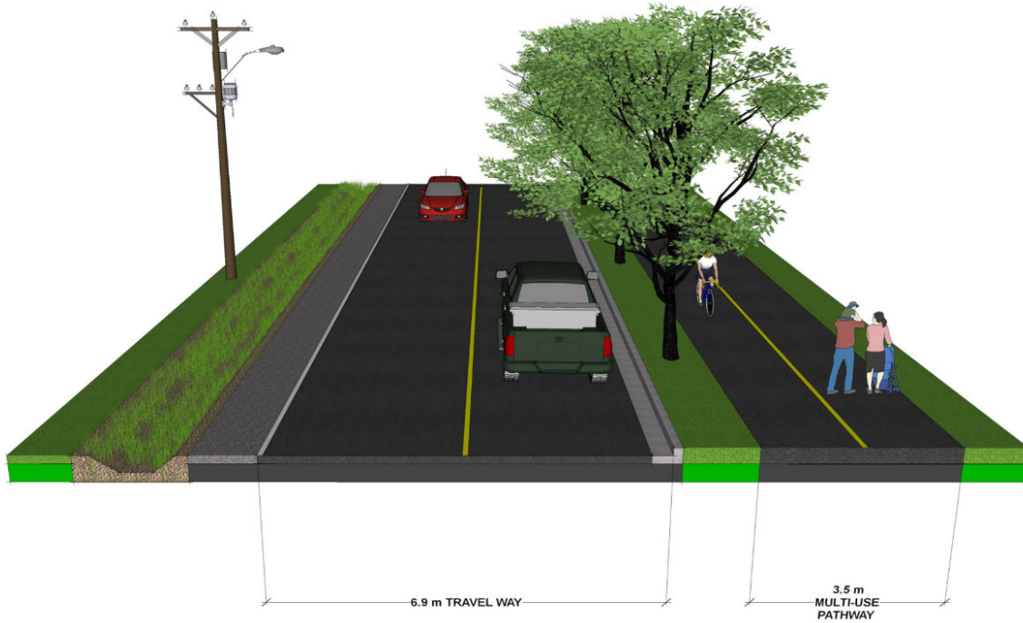
Figure 3-23: Typical Multi-Use Pathway Cross-Section
