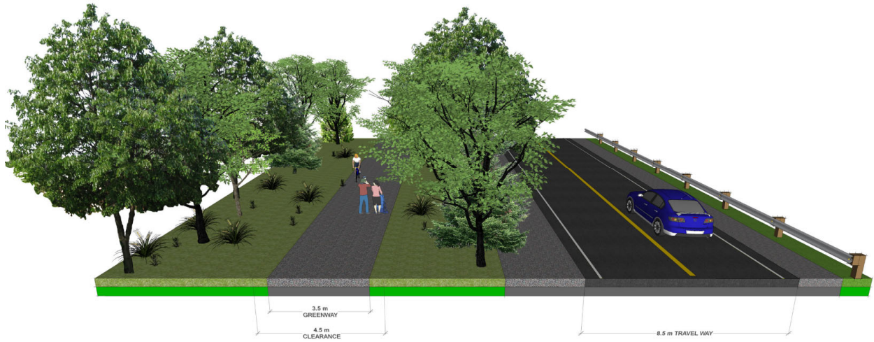
Figure 3-21: Typical Off-Road Greenway Cross-Section
